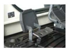
Depress the pedal on the right or left side to extend or retract the boom.
