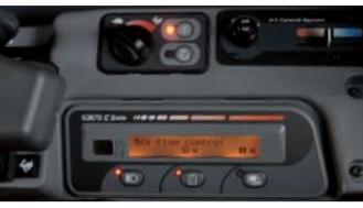
The unique Kubota Intelligent Control System gives you precise control of oil flow according to your needs or the attachment in use.
